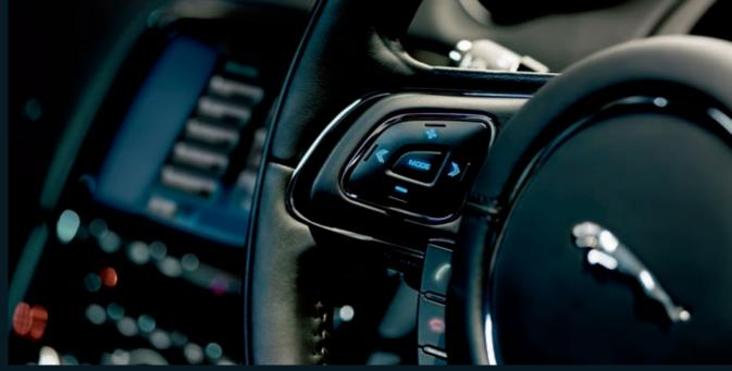
Interactive Controls - 5-way steering wheel mounted controls
