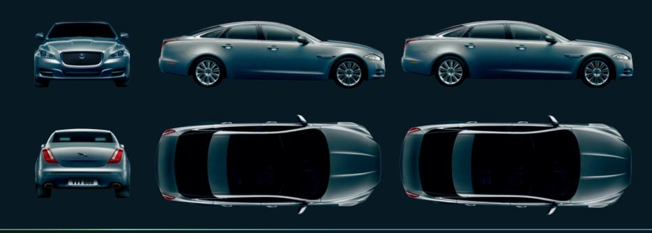
STANDARD WHEELBASE Overall length 5,122mm Overall height 1,448mm Wheelbase 3,032mm Front track 1,626mm
