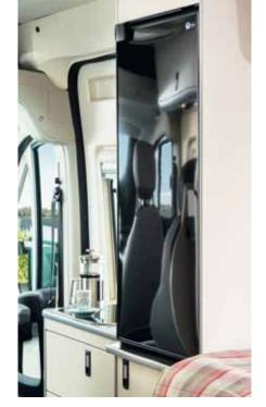
▶ Optionally the refrigerator can be placed above the counter top to gain additional storage space underneath the refrigerator.
