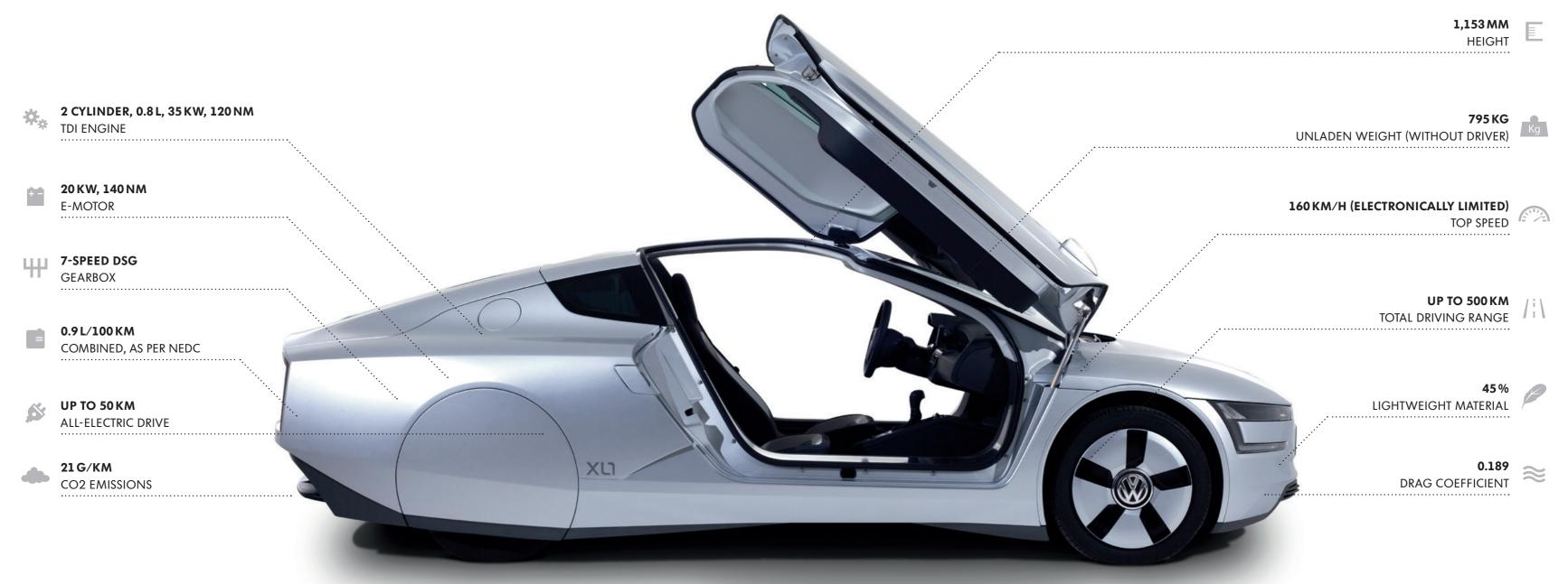
Fuel consumption: 0.9 I/100 km (combined); Power consumption: 7.2 kWh/100 km (combined); CO<sub>2</sub> emissions: 21 g/km (combined); Efficiency rating: A+
