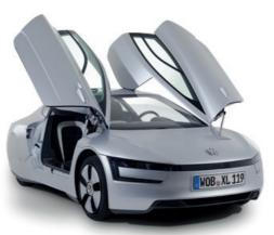
The wing doors extend far into the roof. They do not just swivel upward, but slightly forward as well – which creates an exceptionally large amount of entry and exit space.
