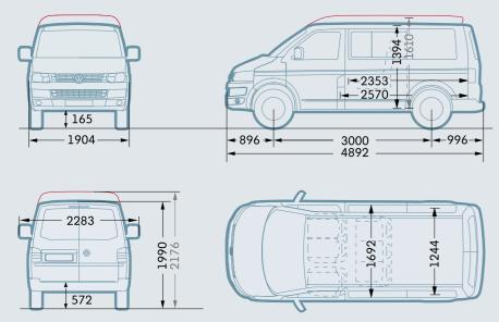
The height measurements listed here may vary by  $\pm$  50mm depending on equipment fitted. Please note vehicle drawings are not to scale
