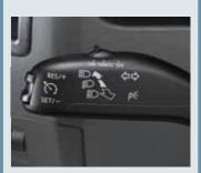
Cruise control Relieve motorway or towing strain by setting your speed with this clever switcl
