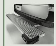
Full-width rear step This strong step with an anti-slip surface, makes loading and unloading easier
