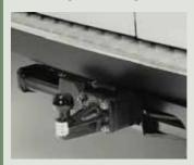
Fit a fixed (or removable) ball or jaw-type and you can haul an extra two tonnes
