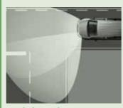
Fog lights with cornering Reduce the risk of accidents by lighting up the road in the direction you're turning
