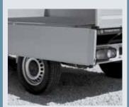
Dropside body – alloy This factory option is made with doubleskinned panels with forged steel hinges
