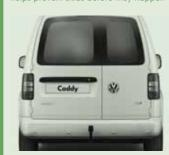
**Opaque asymmetric rear doors**This clever design means that most loads can be accessed by opening just one door
