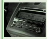
RCD 310 radio / CD player DAB and MP3-compatible with peaker upgrade and AUX-in attack
