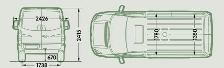
The height measurements listed for dimensions are based on vehicles of standard specification, and may differ by approx ± 40mm depending on equipment fitted. Please note, vehicle drawings are not to scale.
