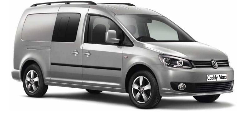
The Caddy Maxi has a load length of 2.25m, so there's even room in the back for a decent-sized step ladder
