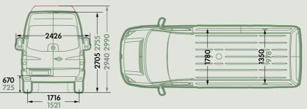
The height measurements listed for dimensions are based on vehicles with standard specification, and may differ by approx ± 40mm depending on equipment fitted. Please note vehicle drawings are not to scale.
