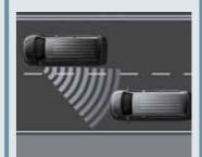
Lane change assist Flashing LED lights in the external mirrors warn of vehicles lurking in your blind spots
