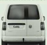
Opaque asymmetric rear doors his clever design means that most loads can be accessed by opening just one door
