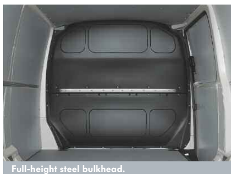
Full-height steel bulkhead.
