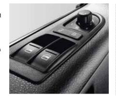
Electric front windows and electrically adjustable mirrors are fitted as standard
