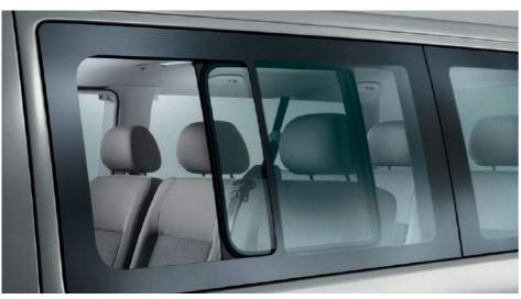
Optional sliding windows in side sliding doors. Available for both driver and passenger side.
