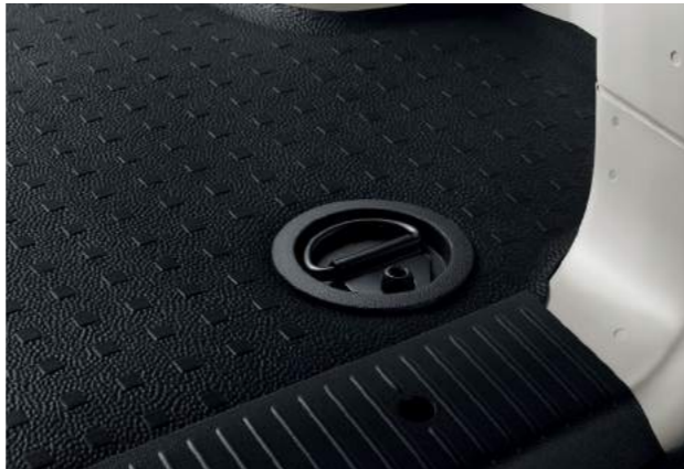
Rubber floor covering with securing points throughout rear passenger area and load compartment.
