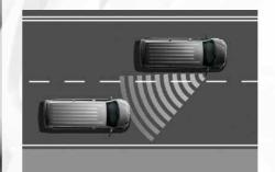
Lane Change Assist<sup>1, 2</sup> has radar sensors to help monitor traffic. When you change lanes, the system warns you via flashing lights in the exterior mirrors if another vehicle is identified within the blind spot.
