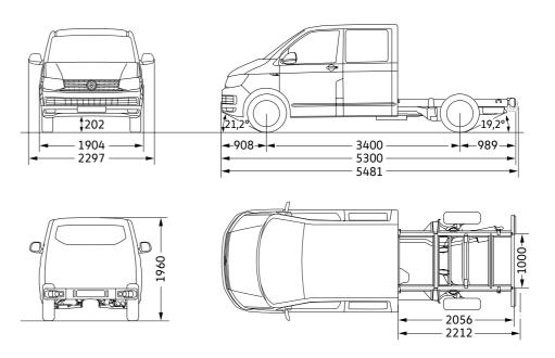
Please note: Vehicle drawings are not to scale. All dimensions in millimetres (mm), unless otherwise stated. The height measurements listed may vary by ± 50mm depending on model and equipment fitted.
