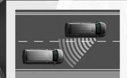
Lane Change Assist<sup>1, 2</sup> has radar sensors to help monitor traffic. When you change lanes, the system warns you via flashing lights in the exterior mirrors if another vehicle is identified within the blind spot.
