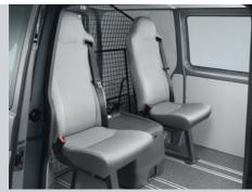
The "Expedition" package. This package offers robust floor rails, reinforced 16" steel wheels with A/T tyres, more pulling power due to shorter gear ratios, and two single seats upholstered in hardwearing "Robust" cloth. The single seats can be adjusted on the floor rails and completely removed if necessary. Three additional single seats can be ordered for the passenger compartment as options. The package can only be supplied for the 103 kW engine version<sup>1)</sup>.
