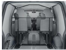
Mesh **partition**<sup>2)</sup>. A roof high, black mesh partition is available as an option. It can be adjusted infinitely on the floor rails between the B and D pillar.
