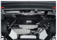
The "Protection" package comprises side sill strips and four different and four different underride guards made of sheet aluminium which protect the underbody from damage, dirt and from making contact with the ground. These underride guards protect the engine and gearbox, the rear axle differential, the main silencer, and the fuel tank.
