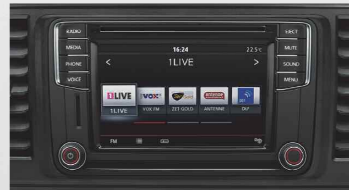
Composition Media DAB+ radio system. The optional Composition Media DAB+ radio system features an increased touch-screen size of 6.33" with proximity sensor, USB port, Bluetooth®, SD card slot, AUX-IN interface, MP3 and WMA compatible CD drive, 4 x 20 watt output with four speakers and a dual tuner with PhaseDiversity for optimum radio reception. App-Connect is available as an option for this system.
