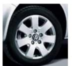
16" Miyato alloys 6.5J x 16 alloy wheels fitted with 215/65 R16 tyres.
