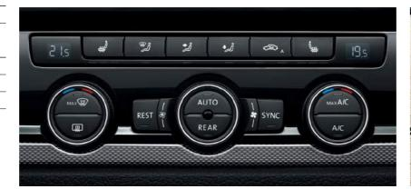
Climatronic three-zone automatic air conditioning and heated seats.
