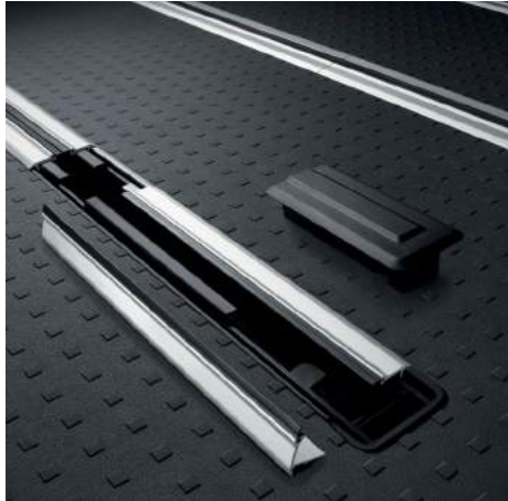
The Caravelle's ingenious floor-mounted rail system shown with optional rubber flooring.
