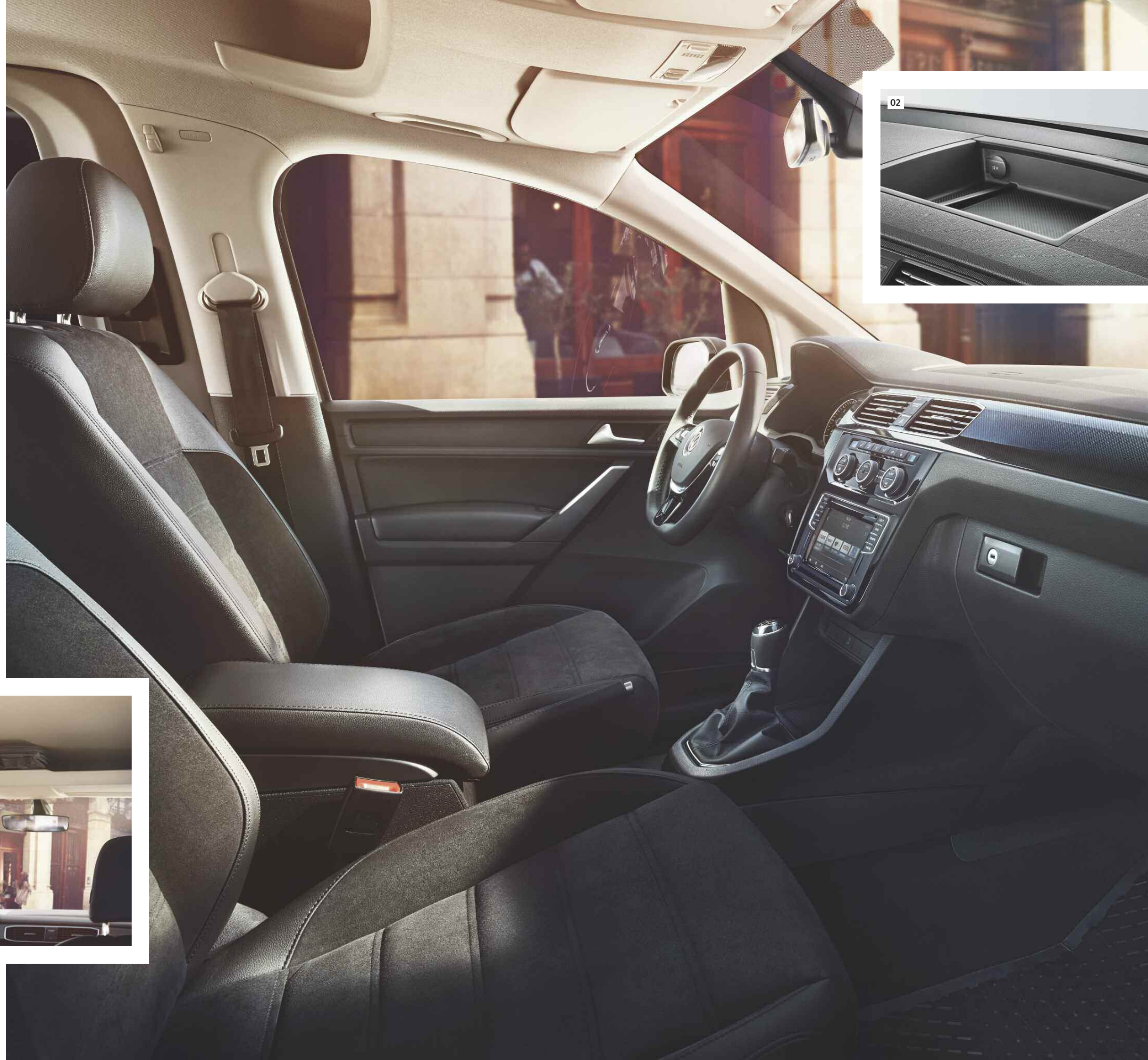
01 Standard above-cab storage shelf. 02 Standard open storage tray with 12v socket.
