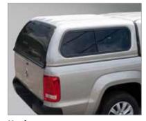
Hardtop In lightweight body-coloured ABS plastic, the hardtop clamps easily to the body. With a foldout passenger-side window, and dual driver'sside sliding window. Can be used with bed liners. Fitted price ex VAT £1.916.67 Fitted price inc VAT £2,300.00
