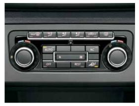
**Climatronic: automatic two-zone air-conditioning** Air conditioning that constantly assesses and corrects the cabin air temperature to keep your vehicle's environment just how you want it
