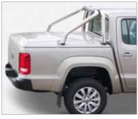
Hard tonneau cover (3-piece) Lockable, weather-resistant lid in durable PC/ABS plastic. Opens on two compressed-gas struts. Three-piece must be combined with the rear styling bar. Available pre-painted in six Amarok colours.
