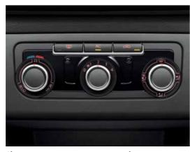
**Climatic: semi-automatic air-conditioning** Makes sure the cabin is supplied with air at a pleasant, consistent temperature of your choice, so you can travel in complete comfort
