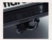
Towing ball and electrics Removable ball-head tow bar (50mm) for 2,800kg trailer loads. With 13-pin electrics. £12.75 Fitted price ex VAT £15.30 Fitted price inc VAT £419.50 Fitted price ex VAT
