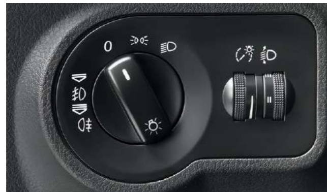
Light control unit with improved activation algorithm
