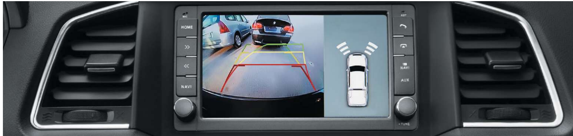
When backing up the vehicle, a color display shows the view from the rear camera with dynamic lines, as well as front and rear parking sensor signals
