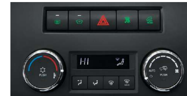
Completely redesigned heating, fans and air conditioning system with climate control functions
