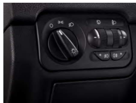
Light control panel
