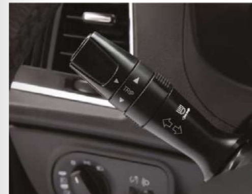
Left-hand under-steering switch with turn signal track mode and on-board computer control
