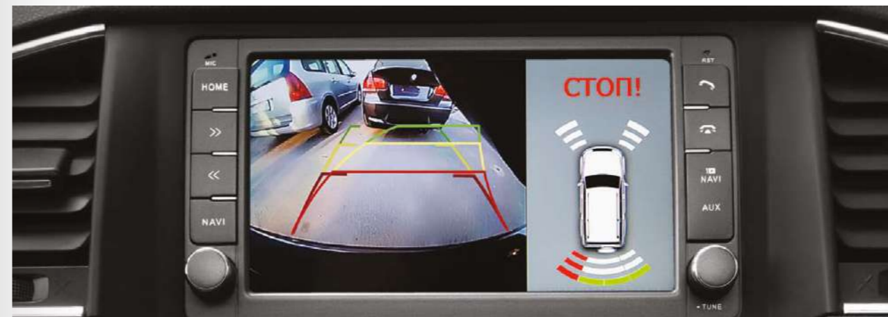
When reversing, a color display shows the view from the rear camera with dynamic guiding lines, and front and rear parking sensor signals
