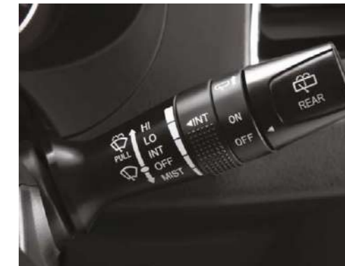
Right-hand under-steering switch with wiper delay control
