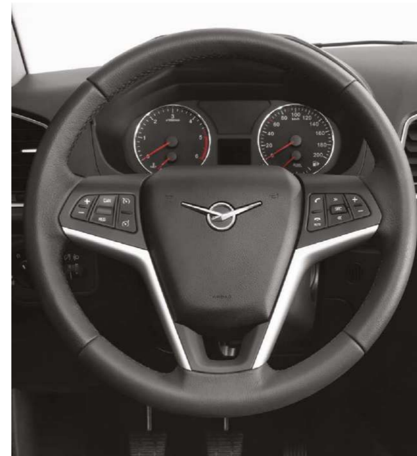
Multifunctional steering wheel with cruise control, speed limiter, multimedia system and loudspeaker system controls
