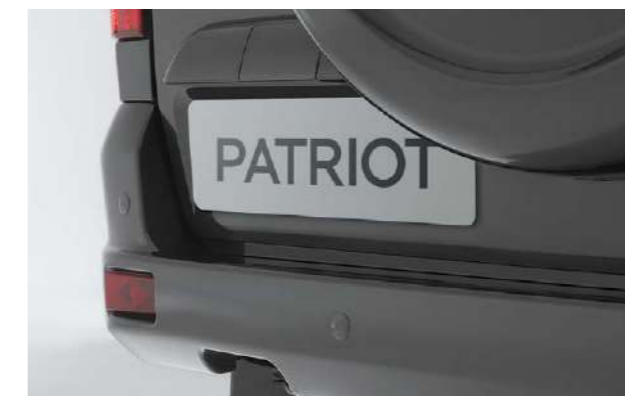
Rear parking sensors on the bumper and rear-view camera in the tailgate handle
