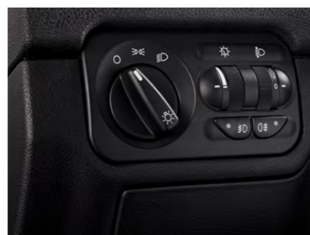
Light control panel
