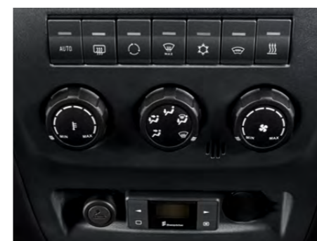
HVAC control panel
