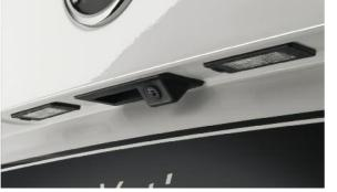
The optional rear-view parking camera, positioned on the tailgate handle, provides a visual of what is behind the car in order to make any parking manoeuvre effortless.
