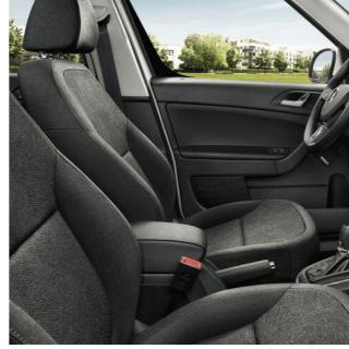
The two outer rear seats in all Yeti models feature **ISOFIX** as standard. The ISOFIX brackets create a fixed link between a child seat and the car's chassis, which is important for ensuring the seat is effectively secured in the event of a collision. ISOFIX can be specified on the front passenger seat too.
