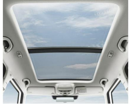
Panoramic sunroof. Standard on Laurin & Klement and optional on SE and SE L. The electrically-operated panoramic sunroof consists of two parts: the front section tilts to provide ventilation but also slides backwards over the rear section, providing fresh air, light and a feeling of vast space.
