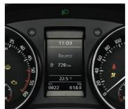
Maxi-DOT comes as standard across the Yeti range. Maxi-DOT, with it's larger display, details fuel consumption, average speed and distance until the fuel tank is empty, and also has the ability to display phone, audio and navigation data too.
