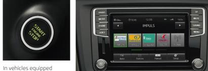
with the optional **KESSY** (Keyless Entry, Start and exit system) the driver can lock and unlock the car as well as start and stop the engine without having to insert or even handle the car key.
