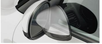
**Door mirrors.** Electrically adjustable and heated door mirrors are standard and come in body colour on Yeti and in matt silver on Yeti Outdoor. Functionality is further enhanced as electrically folding door mirrors with boarding spots are standard on SE L, and Laurin & Klement includes auto-dimming function in the driver's door mirror too.
