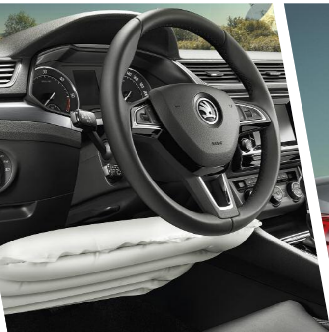
The knee airbag, located under the steering wheel column, protects the driver's knees and shins.
