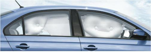
passenger front, side and curtain airbags. Should an impact occur, large-volume airbags activate in conjunction with the front seat belt pretensioners. This will anchor you in the middle of the seat and cushion you to reduce injury.
