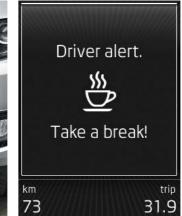
**Fatigue sensor.** Standard from SE is a Driver fatigue sensor. This monitors the movement of the driver through the steering wheel and if the driver begins to display signs of tiredness, the car will audibly alert the driver with a tone and show a break recommendation alert on the Maxi DOT.
