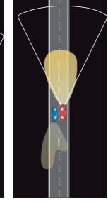
The oncoming vehicle has left more than a second, so the car switches to high beam again.
