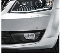
Bi-Xenon lights. The optimal illumination of the Bi-Xenon lights is enhanced by the AFS which changes the light setting depending of the car's speed and weather conditions. Bi-Xenon headlights provide 2.5 times the illumination of halogen headlights.
