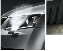
Telescopic front headlight washers. Standard on Elegance, optimise your front lights' range by keeping the front panels clean of dirt and debris.
