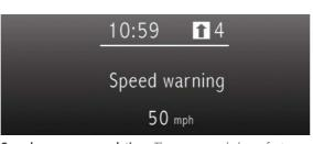
**Gear change recommendations.** The recommended gear feature on the trip computer or Maxi-dot display shows the driver whether the gear they are in is appropriate or whether they need to change
