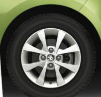
14" Apus alloys 5J x 14" & temporary spare steel wheel
