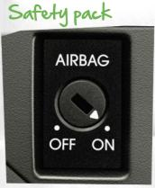
City-Safe with ESC and Passenger airbag Switch-off function
