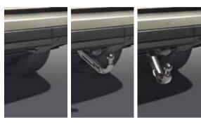
Electrically Deployable Tow Bar VPLGT0081, VPLGB0108, VPLGT0109, VPLGT0108
