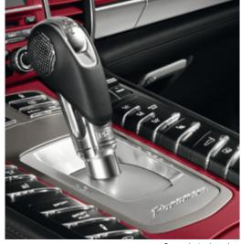
PDK gear selector in aluminium
