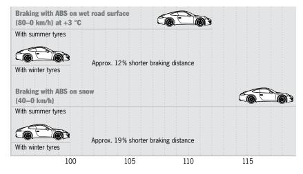
Braking distance in % (measured with the use of tyres conforming to the Porsche specification). Braking distances optimised by the use of Porsche winter tyres. Absolute values may vary.
