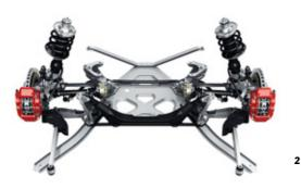
In 'Sport' mode, the suspension is set to a harder damper rating. On uneven roads, PASM immediately switches to a softer rating, thereby improving contact between the tyres and the road. When the road surface improves,
