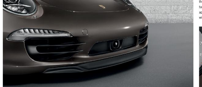
Radar sensor of adaptive cruise control
