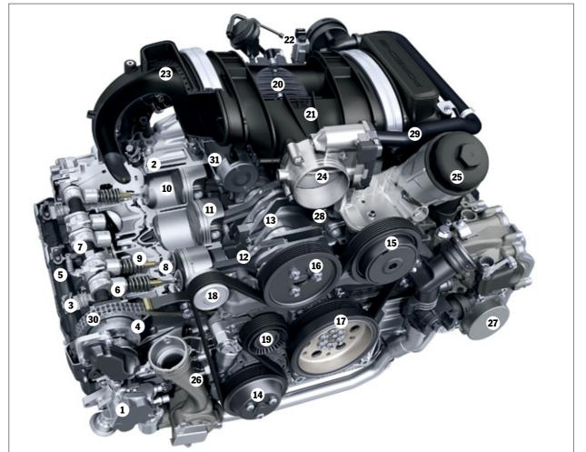
Engine cross section: 3.8-litre boxer engine
