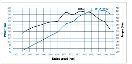
911 Carrera S models: 294 kW (400 hp) at 7.400 rpm, 440 Nm at 5.600 rpm
