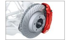
Standard brake system on the 911 Carrera S models
