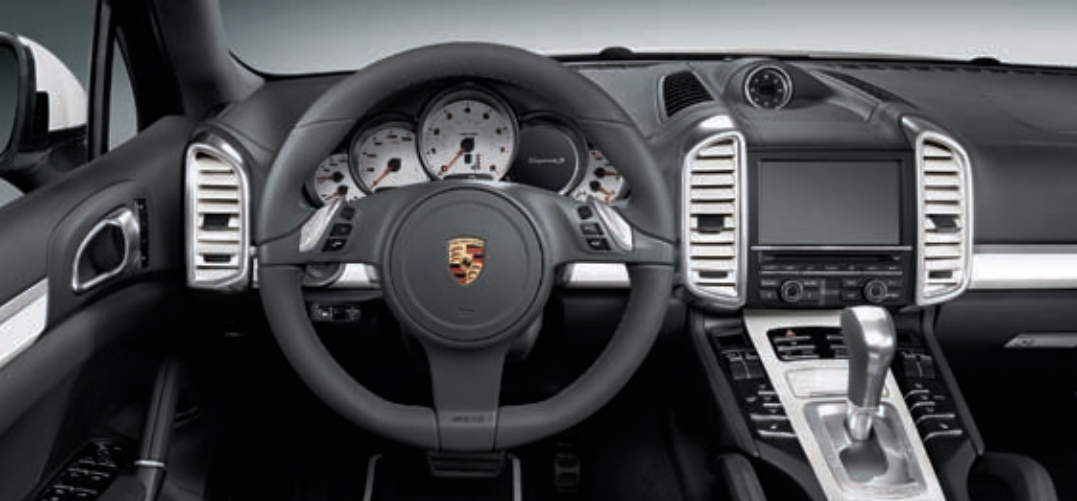
Interior package painted, air vent slats painted, instrument dials in white
