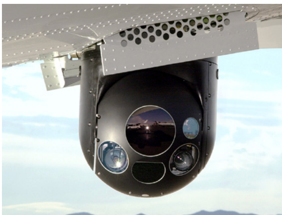
The retractable electro-optical and infrared sensor deploys quickly in flight.
