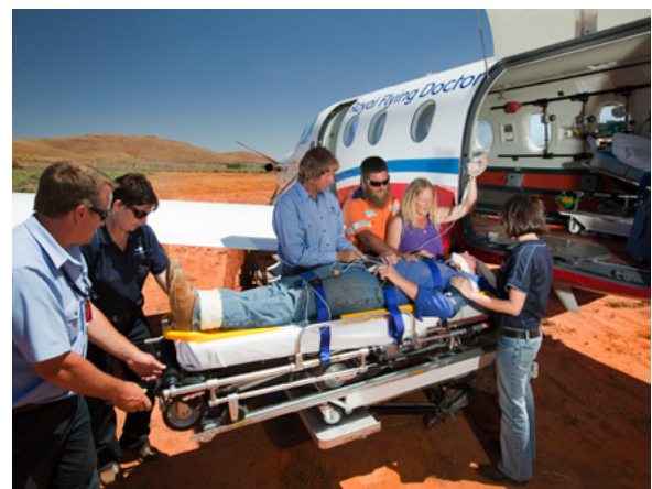
The large cargo door and patient loading system provides unparalleled cabin access for medevac operations.
