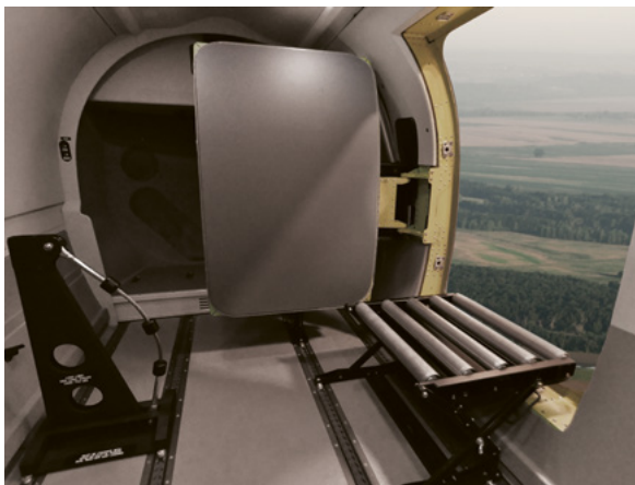
An optional integrated utility and jump door increases the number of roles while retaining the standard cargo door functionality.
