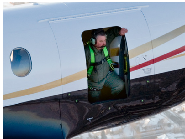
When jump or drop operations are completed, the PC-12 is re-pressurised to climb back to altitude for high-speed performance.
