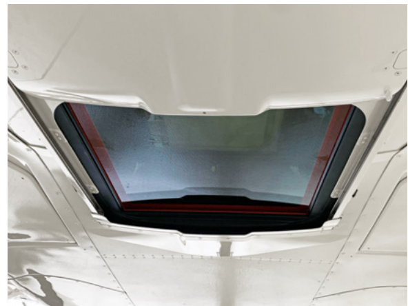
The two hatches can be opened in flight enabling scanning and photography at the same time.
