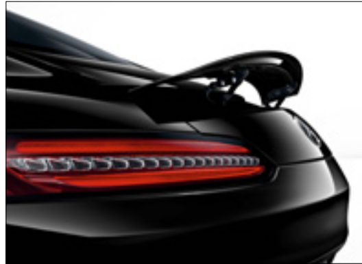
Rear aerofoil – electrically extending
