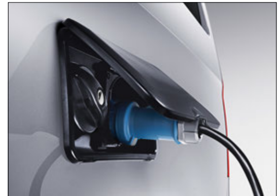
External connections for power and fresh water
