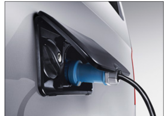
External connections for power and fresh water
