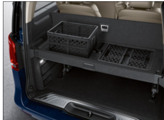
Load compartment divider with two folding boxes
