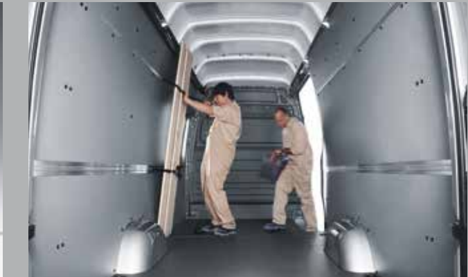
Flexible load-securing and cargo-retention system. Optional lashing rails in the floor, sidewalls and roof frame as well as tensioning straps for the lashing rails are available to secure loads.
