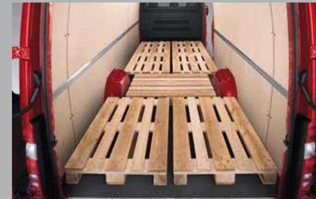
Load compartment. Near-vertical inner walls, minimal wheel arches and a payload of up to 2695 kg allow the available space to be used to the full.
