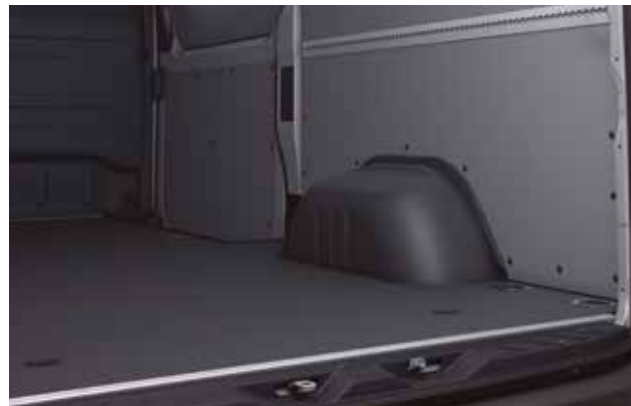
The even surface of the weight-optimised plastic floor facilitates use and maintenance of the load compartment and offers weight savings in the order of 18.5 kg in comparison to the standard wooden floor. 2
