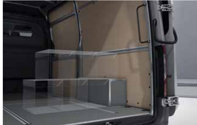
The wood trim on the wheel arches facilitates loading of the load compartment and protects the metal panelling from damage.
