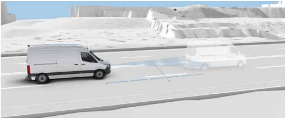
Active Distance Assist DISTRONIC allows the driver to set and maintain a safe distance from the vehicle in front, particularly useful for motorway driving or in stop-and-go traffic.
