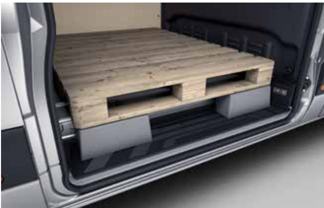
The pallet support in the step of the sliding door stabilises loads in the door area and is particularly useful when transporting Europallets or crates.
