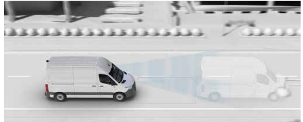
Standard Active Brake Assist can help to avoid accidents with vehicles ahead and with crossing pedestrians or to mitigate the effects of an accident using autonomous emergency braking technology.
