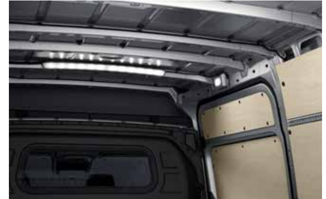
The two LED light strips under the roof illuminate the load compartment, for improved visibility inside when loading and unloading the vehicle.
