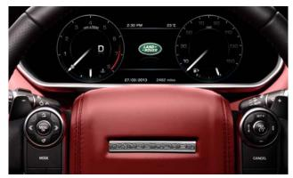
Full Thin Film Transistor (TFT) Instrument Panel
