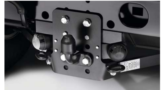
'S' Type Towing Electrics† LR005921 – (shown above, left-hand side) For use when additional trailer power is required. Capable of supplying interior lighting and equipment power including fridge feed and battery charging. Please note: Not compatible with standard fitted 12N sockets. Must be used in conjunction with 'N' Type Towing Electrics LR005920. 'N' Type Towing Electrics† LR005920 – (shown above, right-hand side) Provides power for rear trailer lighting including rear lamps, brake lamps, direction indicators and high intensity fog lamp(s). Can also power a Lighting Board.
