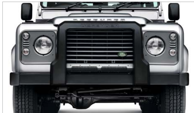
A-Frame Protection Bar – Non winch version VPLPP0060†
