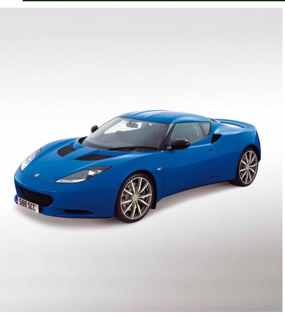
The Evora S blends the sublime handling attributes of the Lotus Evora with the surging linear power of a supercharged V6 engine. Delivering even more attitude, the forced induction power plant delivers 345 hp and 295 lbft of torque. There's no appreciable weight gain: at 1,437 kg the Evora S is still lightweight, muscling from 0 to 60 mph in 4.4 seconds, powering to its 178 mph maximum.
