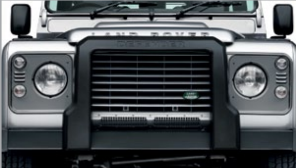
A-Frame Protection Bar – non winch version - VPLPP0060* A-Frame Protection Bar – winch version (not shown) - VPLPP0061* Manufactured from durable polymer, suitable for models with or without air conditioning. *Compliant to EEC Directive 2005/66.
