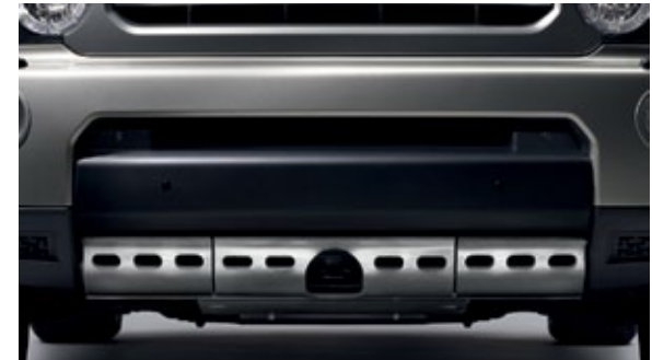
Underbody Protection (non winch version) VPLAP0094
