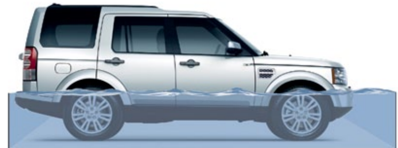
Wading Depth Maximum wading depth 700mm (27.56 in.) Normal wading depth 600mm (23.62 in.)
