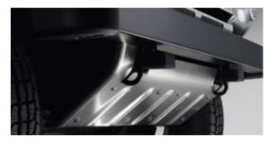
**Ribbed Aluminium Undershield** LR008247 Helps to provide under-engine protection when driving off-road.
