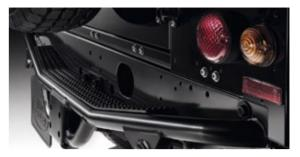
Rear Step Bumper Makes access to the loadspace easy as well as helping to provide added protection from minor knocks, and also incorporates a dual height tow bracket.
