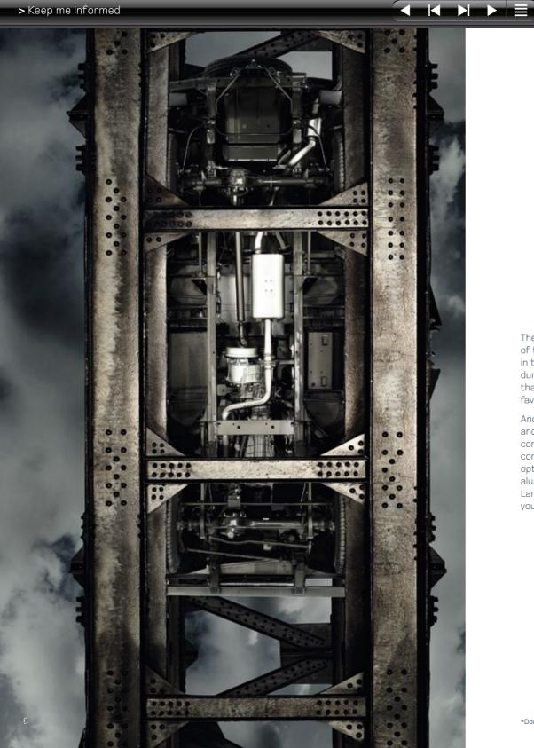
There are some things that'll never need improving. Defender's chassis is one of them. Immensely strong, it is probably the single most important component in the vehicle's design architecture and contributes to its strength, versatility, durability and capability. The box section, ladder frame design is far stronger than an open channel design and more adaptable than the unibody design favoured by many of its competitors.
