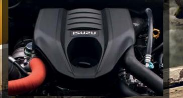
Isuzu 4JJ1-TC Hi-Power turbo diesel engine offers a maximum torque output of 430Nm and 130kW of power
