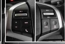
All LS-models<sup>^</sup> are equipped with steering whee cruise, audio and Bluetooth<sup>®</sup> function controls
