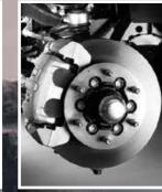
Large front brakes with ventilated disc
