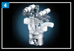
Sophisticated engine head; cam-to-valve roller bearings and variable swirl action gas flow
